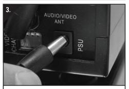
Connect the Power Supply Unit (PSU) to the socket labelled 'PSU' on the Receiver.
