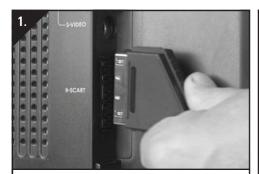
Locate a vacant SCART socket on the back of your receiving TV and insert the DigiSender® SCART cable.
