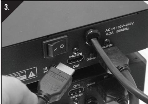
3. Use one of the included HDMI cables and connect it to the socket labelled 'HDMI Out' on the back of the DigiSender® Transmitter and the HDMI Input on your main TV.
