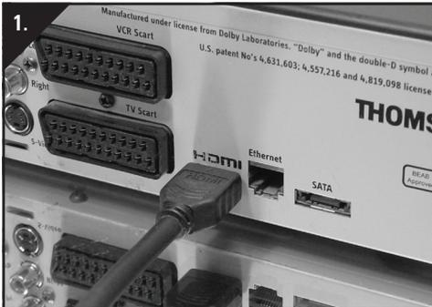
1. Identify the HDMI cable connecting your source device (e.g. HD Satellite receiver) to your main TV.
