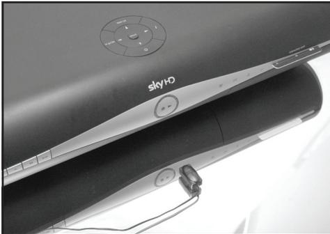
**Position 1:** Place the IR Emitter facing the remote control sensor on the front of your source device (e.g. HD Satellite receiver).
