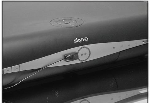
**Position 2:** Use the included sticky pad to stick the IR emitter to the front of your source device, near to, and facing, the remote control sensor.
