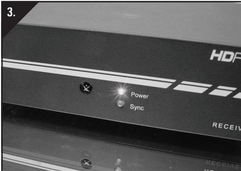
A green LED on the front of the DigiSender® Receiver will illuminate to indicate that the Receiver is powered up.
