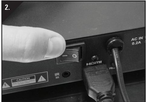
Connect the DigiSender® Receiver power cable to an available mains power socket and switch on at the back.
