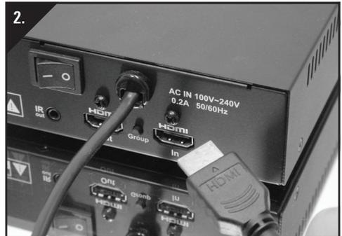
2. Disconnect this cable from the TV and connect it to the socket labelled 'HDMI In' on the back of the DigiSender® Transmitter.
