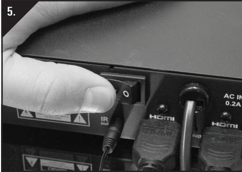
5. Connect the DigiSender® Transmitter power cable to an available mains power socket and switch on at the back.
