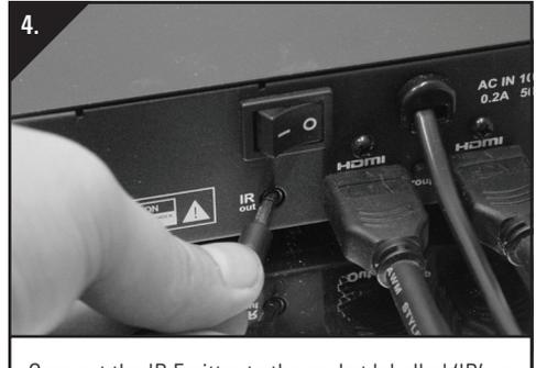
4. Connect the IR Emitter to the socket labelled 'IR' on the back of the DigiSender® Transmitter and place the IR Emitter facing the remote control sensor on the front of your source device (e.g. HD Satellite receiver).
