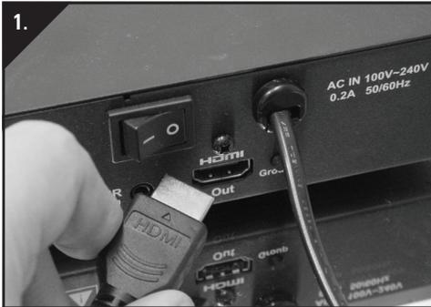
Use the remaining HDMI cable and connect it to the socket labelled 'HDMI Out' on the back of the DigiSender® Receiver and the HDMI Input on your receiving TV.
